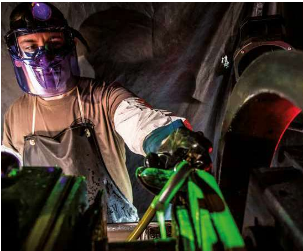
NDI Technician of the 108th Maintenance Squadron, analyzes a part of the KC-135R Stratotanker aircraft at Joint Base McGuire-Dix-Lakehurst, N.J., using a Labino UVG5 headlight.
